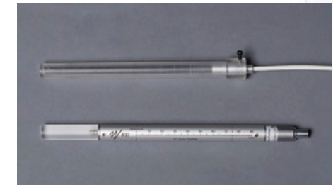
CT dosimetry with an ionization chamber and a solid state detector
