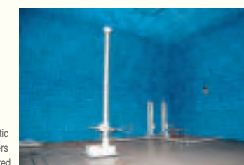
Large test facility where electromagnetic noise at a distance up to 10 meters from the equipment can be measured
