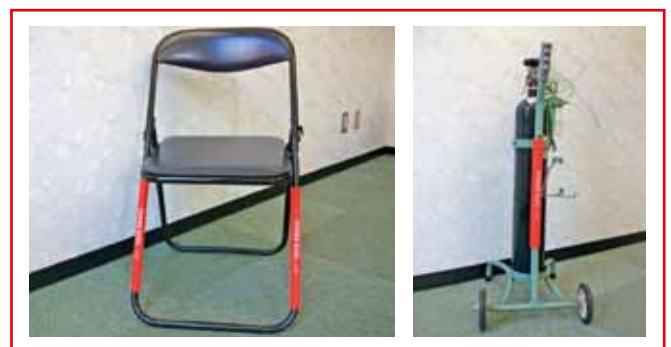
Red marking (for devices that must not be brought into the MRI room)
